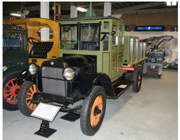
1925 1½-ton six-cylinder REO Speed Wagon, which was introduced with a load capacity of 2,500 lbs.
