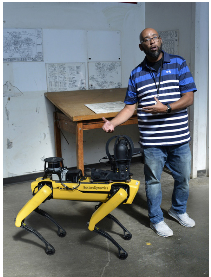
Astro with building superintendent and tour leader Troy Guy. Astro is outfitted with a rotating high definition digital cam in a roll cage and sensing equipment for thermal and acoustic inspections.
