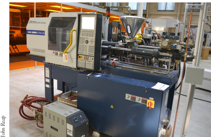
Van Dorn-Demag Extra 28-series, 28-ton clamping-force injection molding machine at the NPIC. The stainless steel material hopper is on the right.
