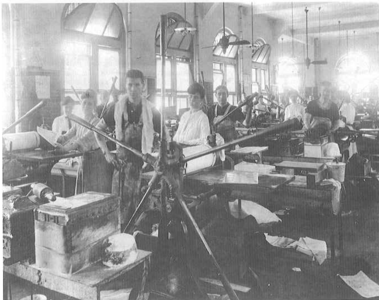
Hand-powered flatbed spider press in the original BEP building, ca. 1904; the pressmen are aided by female printers' assistants. Courtesy Bureau of Engraving and Printing.
